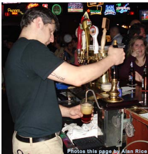
Lazy Boy Saloon used to have cask ale up until 2005 when that was replaced by two fake “hand-pump simulators,” above, that look like real cask engines but simply serve keg beer on low gas pressure. We’re glad to see they have since re-installed two cask engines.
