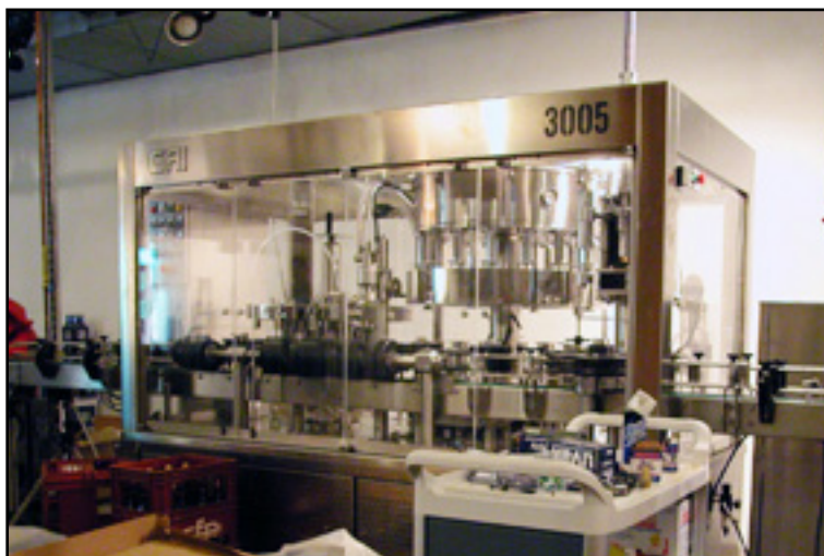
Empty bottles enter from the left. They are rinsed, evacuated and filled.
